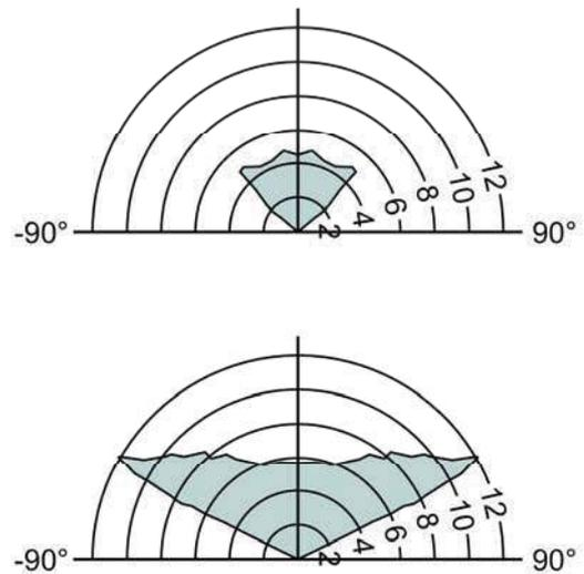
Figure 10: Advisory plots regarding parametric rolling with  $PRFI \geq 4$  in the grey zones for Fidelio in design load condition, ship speed between 0 and 12 knots, true wind 20m/s, significant wave height 5m, mean period of 8s, wind and waves coming from 0°, with (top) and without (bottom) aerodynamic roll damping.
