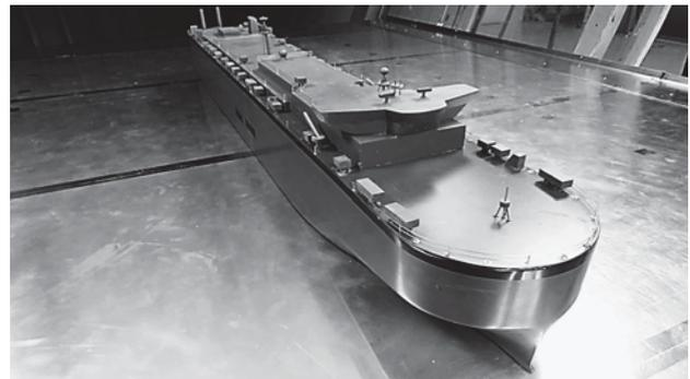
Figure 5: Wind tunnel model of PCTC Fidelio
