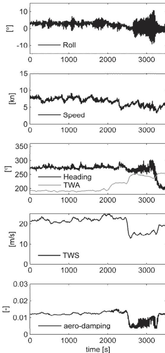
Figure 9: Time series of Fidelio’s roll motions, speed, heading, true wind angle (TWA), true wind speed (TWS) and estimated aerodynamic damping from the event in 2011.
